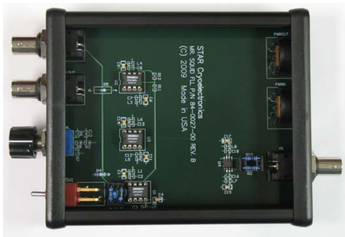
Interior view of the Mr. SQUID Flux-Locked Loop box.
